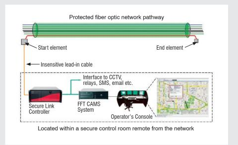
At the heart of the system is the intelligence built into the FFT Secure Link controller. In parallel with detection, advanced signal processing techniques are used to identify and eliminate environmental nuisance alarms such as building noise, vehicle traffic and weather effects.
