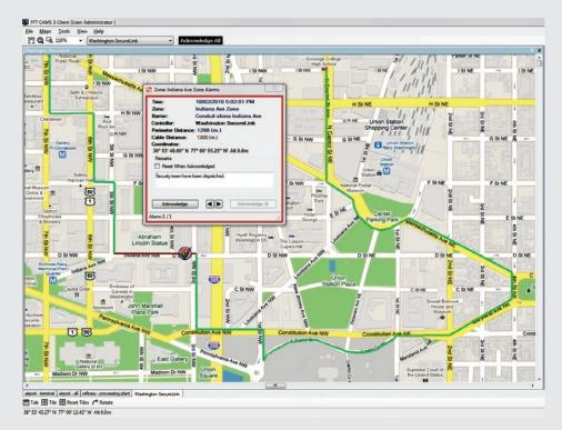
Connecting FFT Secure Link to FFT CAMS™ enables the location of interference and intrusion alarms to be displayed on an intuitive map based user interface and logged into a secure database.
